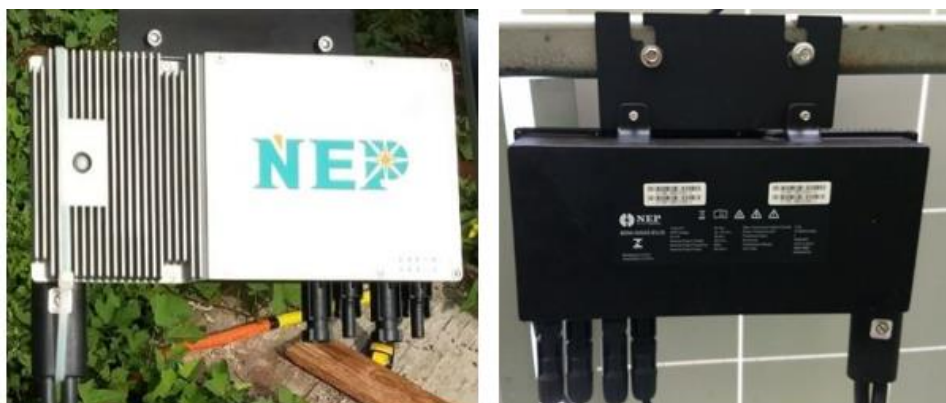
Figura 19 – Microinversor, fabricante Northern Electric (NEP), modelo BDM-300X2-EU-D
