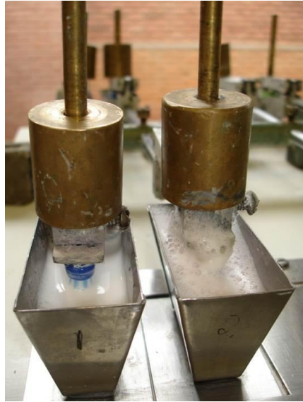
Figure 7. Three-body abrasion test – Mechanical degradation
